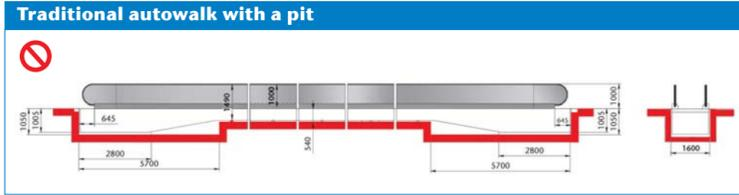
KONE InnoTrack™ autowalk can be installed on a finished floor, it does not require a pit and can be located on any floor.
