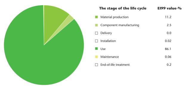
The most significant environmental aspects of the escalator are fossil fuels (particularly hard coal and crude oil) and air emissions (particularly carbon dioxide, nitrogen oxides, sulfur oxides and particulates) according to the CML-Impact
